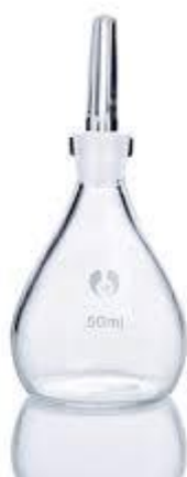
Figure 8: Schematic view of Pycnometer (RD bottle)
