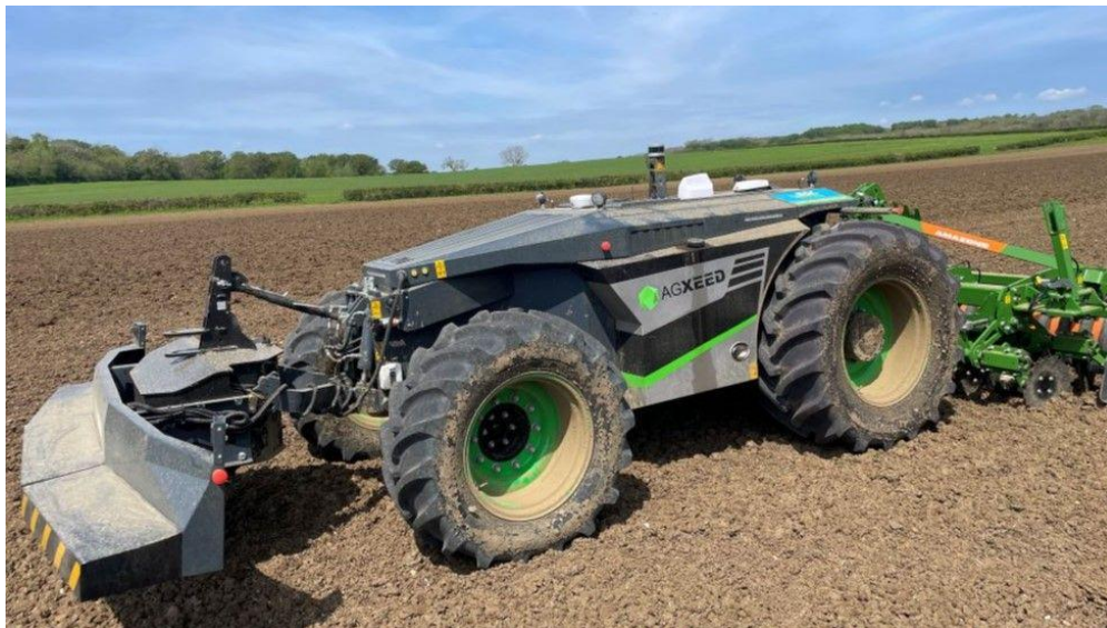
Figure 4: Autonomous robot tractor with AI
