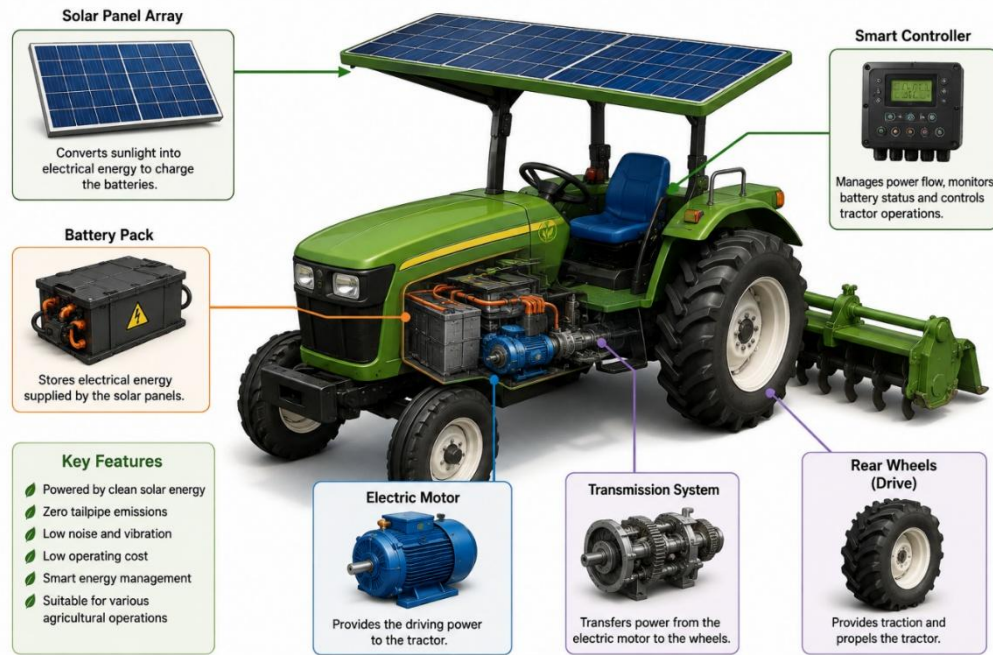
Figure 3: Conceptual Layout of a Solar-Powered Electric Tractor
