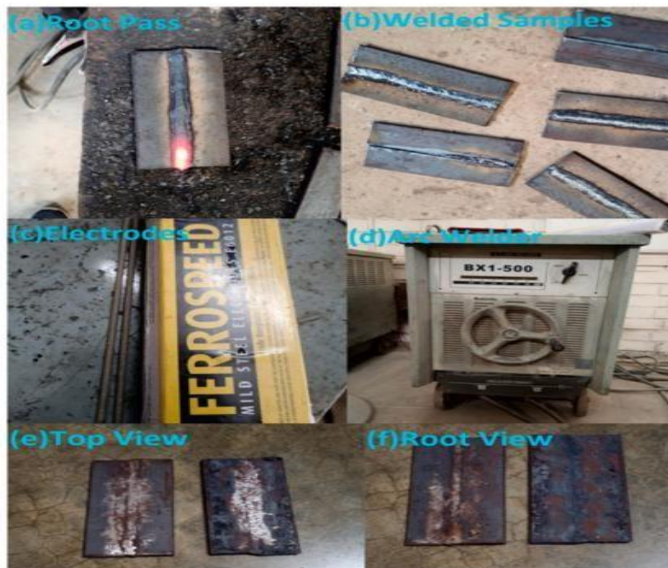
Figure 1: (a) root pass, (b) welded samples (c) electrodes used, (d) arc welder, (e) top view of the plate, (f) root view of the plate.
