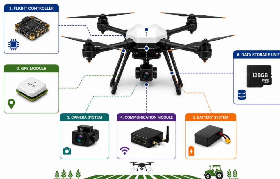
Figure 3: Major components of an agricultural drone system
