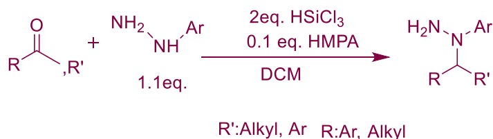
Scheme 3 Synthesis of N-Arylhydrazines
