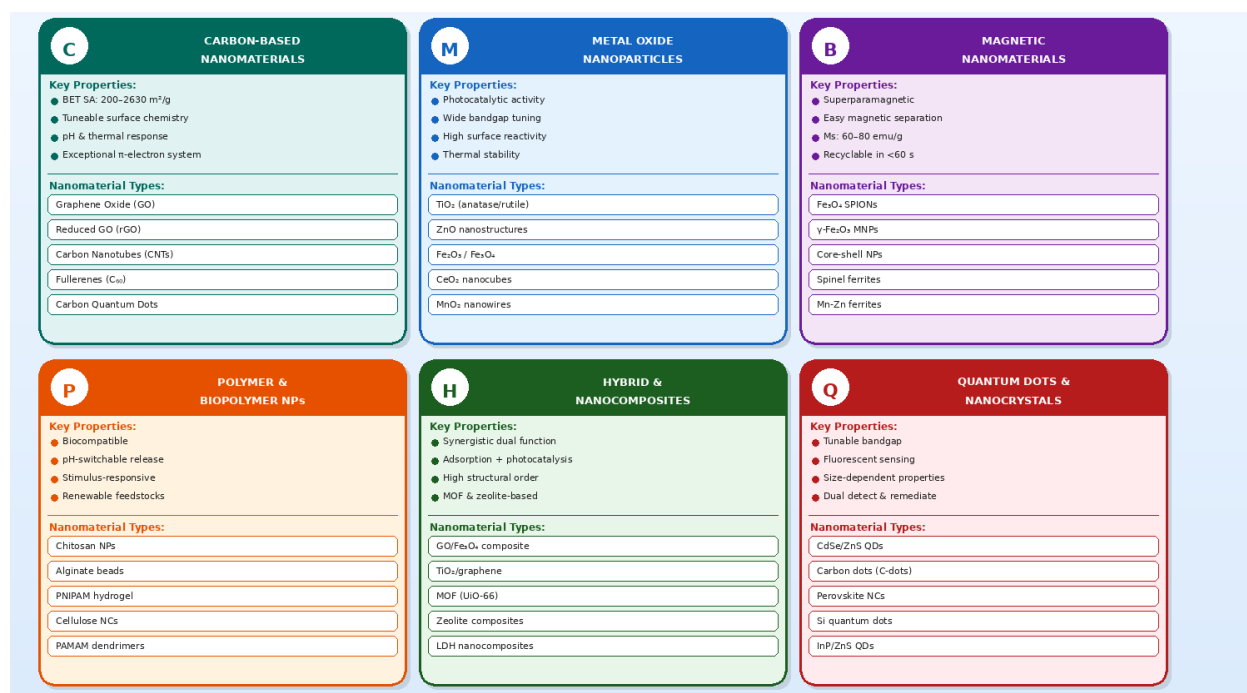
Figure 1: Classification of smart nanomaterials used in environmental remediation. The six principal categories are distinguished by their compositional basis and dominant remediation mechanism. GO = graphene oxide; CNTs = carbon nanotubes; MOF = metal-organic framework; MNPs = magnetic nanoparticles; NPs = nanoparticles.
