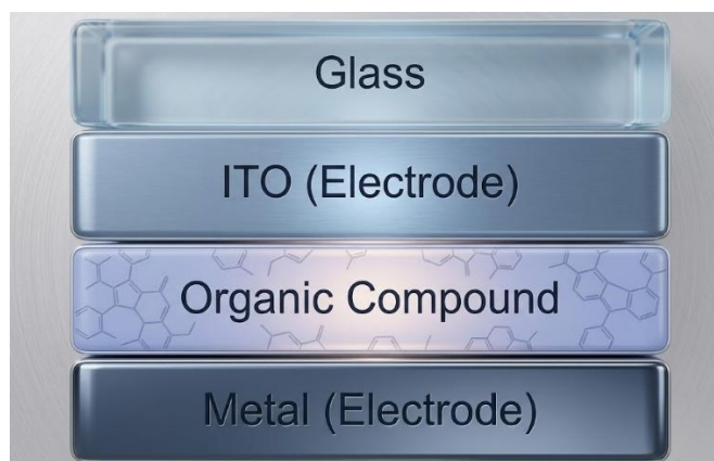
Figure 1: Construction of Single Layer Organic Solar cell
