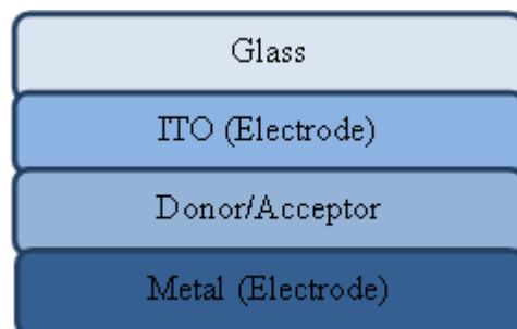
Figure 3: Construction of Bulk Heterojunction Solar Cell
