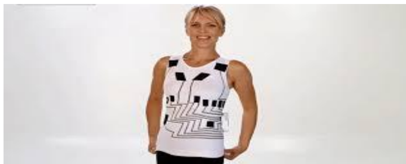
Figure 4: Washable T-shirt with sensors to read vital signs
