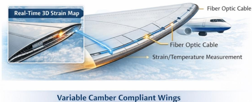
Figure 3: Embedded Fiber Optic Sensors for Structural Health Monitoring
