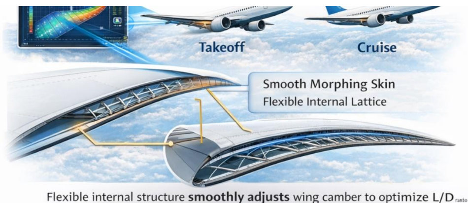
Figure 5: Variable Camber Compliant Morphing Wing Structure
