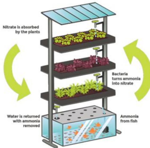
Figure 4: Mechanism of Aquaponic System
