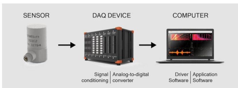
Figure 2: Data acquisition system block diagram
