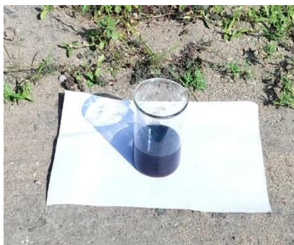
Figure 5.11: Mixture of MB solution with Ferrite particles expose to sunlight light.
