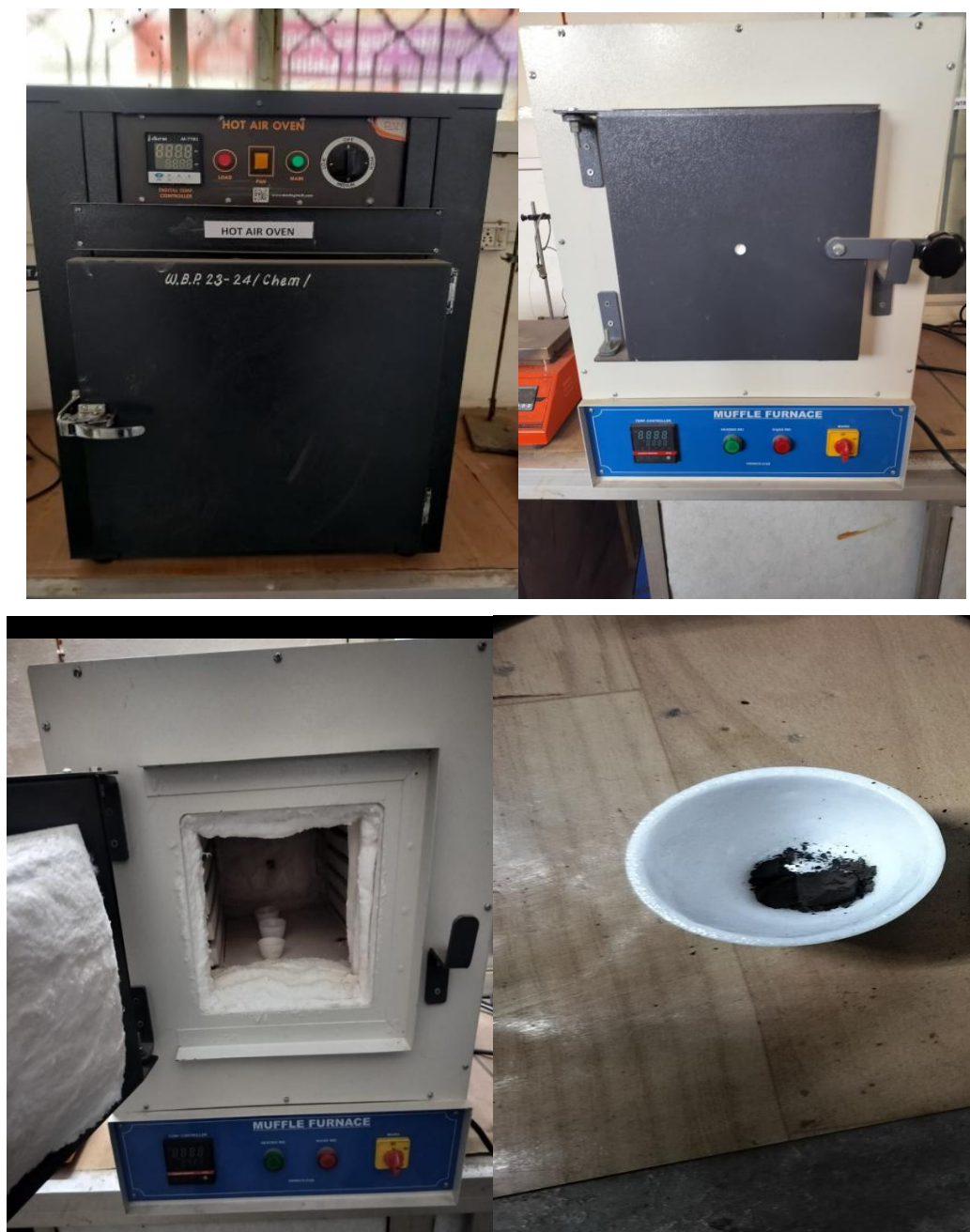
Figure 3.3: For Pre heating and calcination of sample at 800 °C
