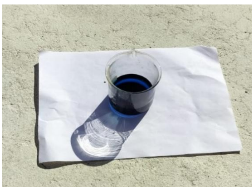
Figure 5.17: Mixture of MB solution with Ferrite particles expose to sunlight light.
