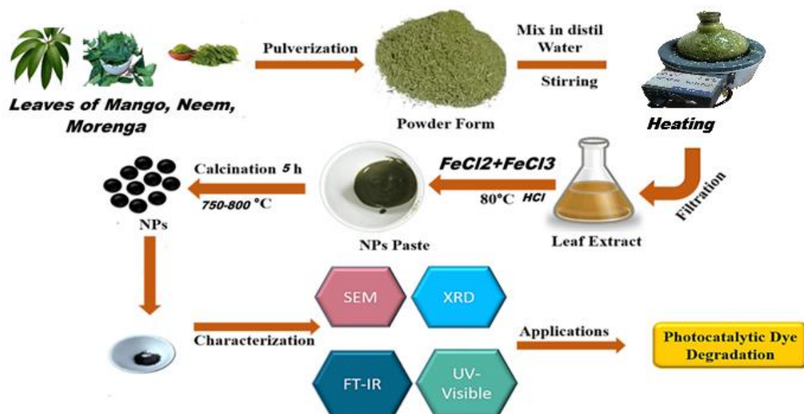
Figure 3.4: Process of Green synthesis of Nano ferrites from Different leaves
