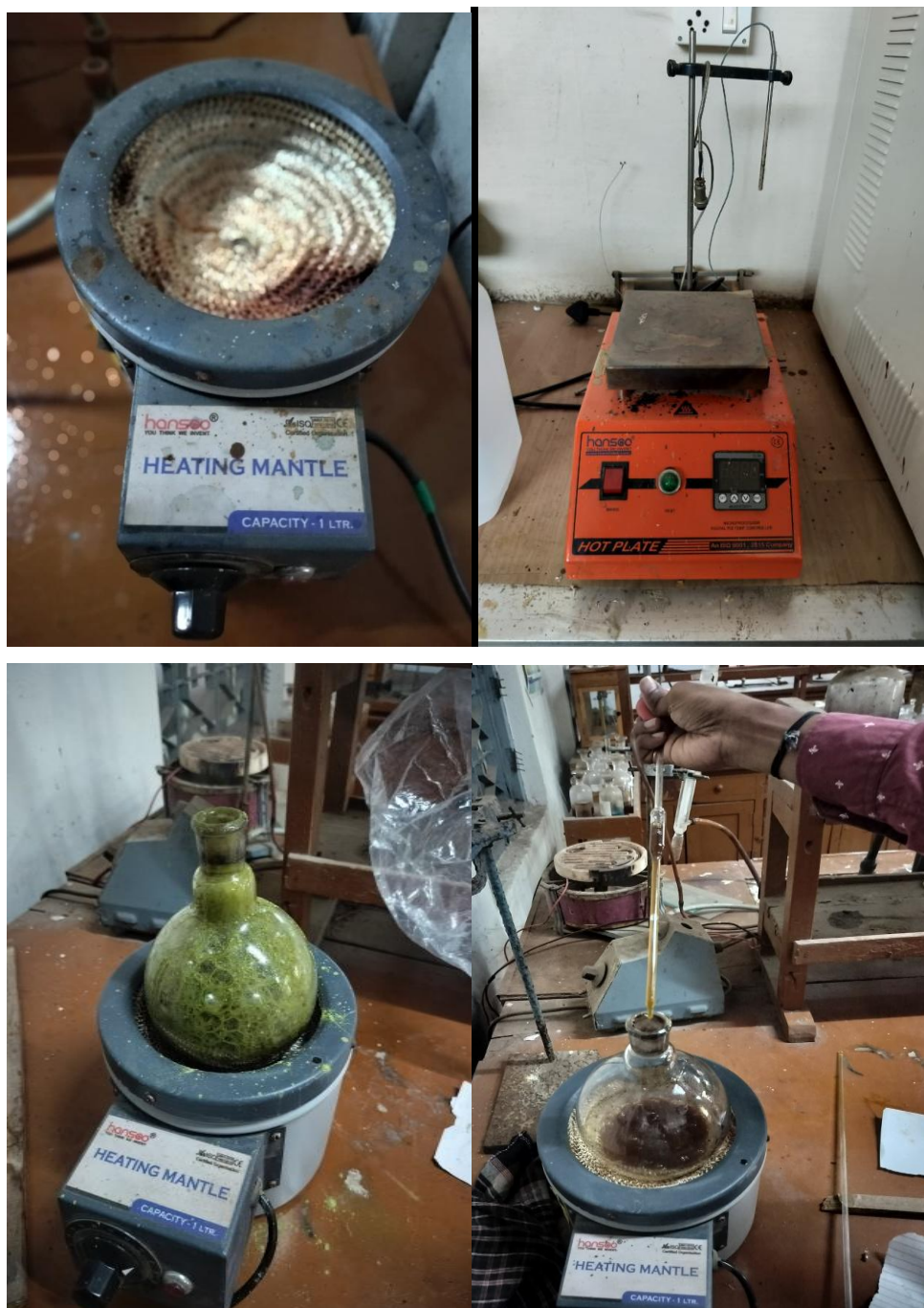
Figure 3.1: Synthesis of Green Ferrite at constant temperature
