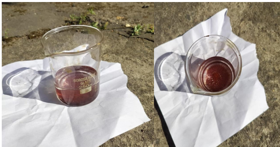
Figure 5.13: Degradation of MB under sunlight after 6 hours.
