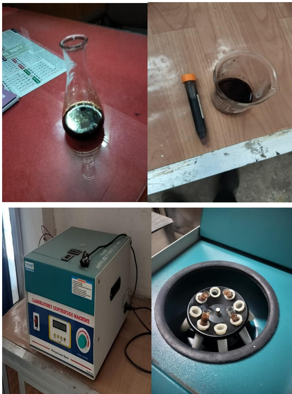
Figure 3.2: Separation of Nano Ferrite particles by using Centrifuge.
