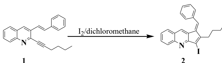
Scheme 1: Synthesis of 3-iodo-1H-cyclopenta[b]quinoline from enyne 1 using I 2 .
