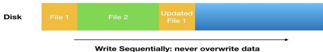
Figure 4.3: Sequential write mechanism in a Log-Structured File System (LFS).
