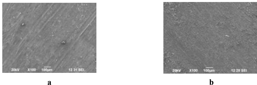
Figure 6: SEM images of mild steel specimen immersed in 1M H 2 SO 4 in the absence and presence of inhibitor MBTP at 1000 ppm
