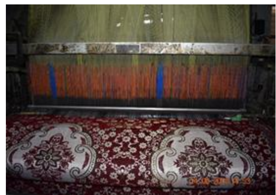
Plate 2: Weaving of Fabric on Power Loom with Jacquard Attachment
