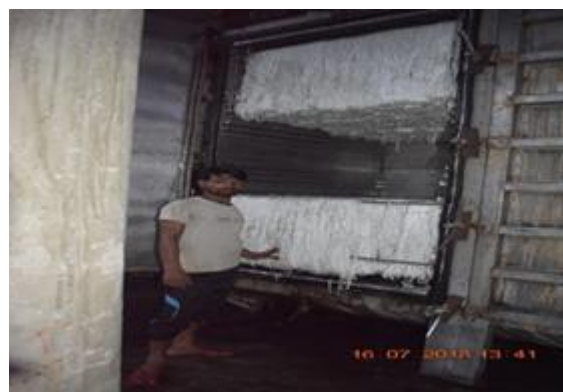
Plate 3: Cabinet Dyeing of Yarns in Units with Dyeing in-house Facility or Separate Dyeing Units
