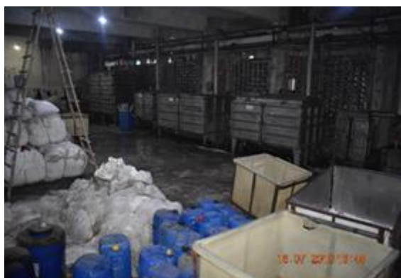
Plate 3: Cabinet Dyeing of Yarns in Units with Dyeing in-house Facility or Separate Dyeing Units
