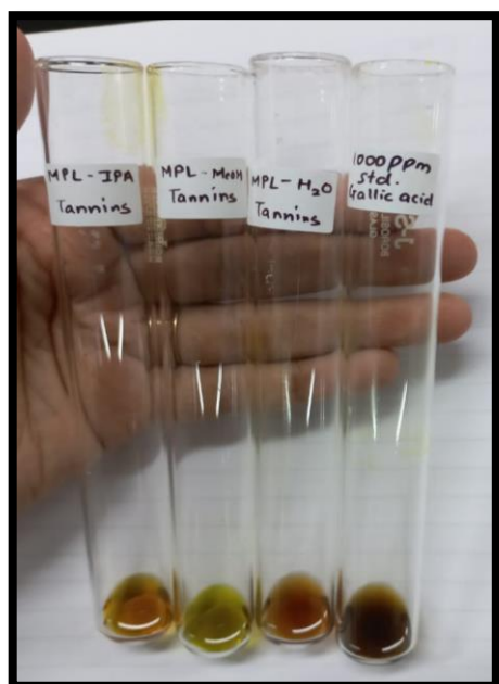
Figure 1: Qualitative FeCl 3 test showing the presence of tannins when compared to standard Gallic acid
