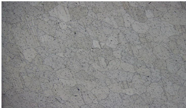
Figure 7: Base metal microstructure of the aluminum alloy 6063.
