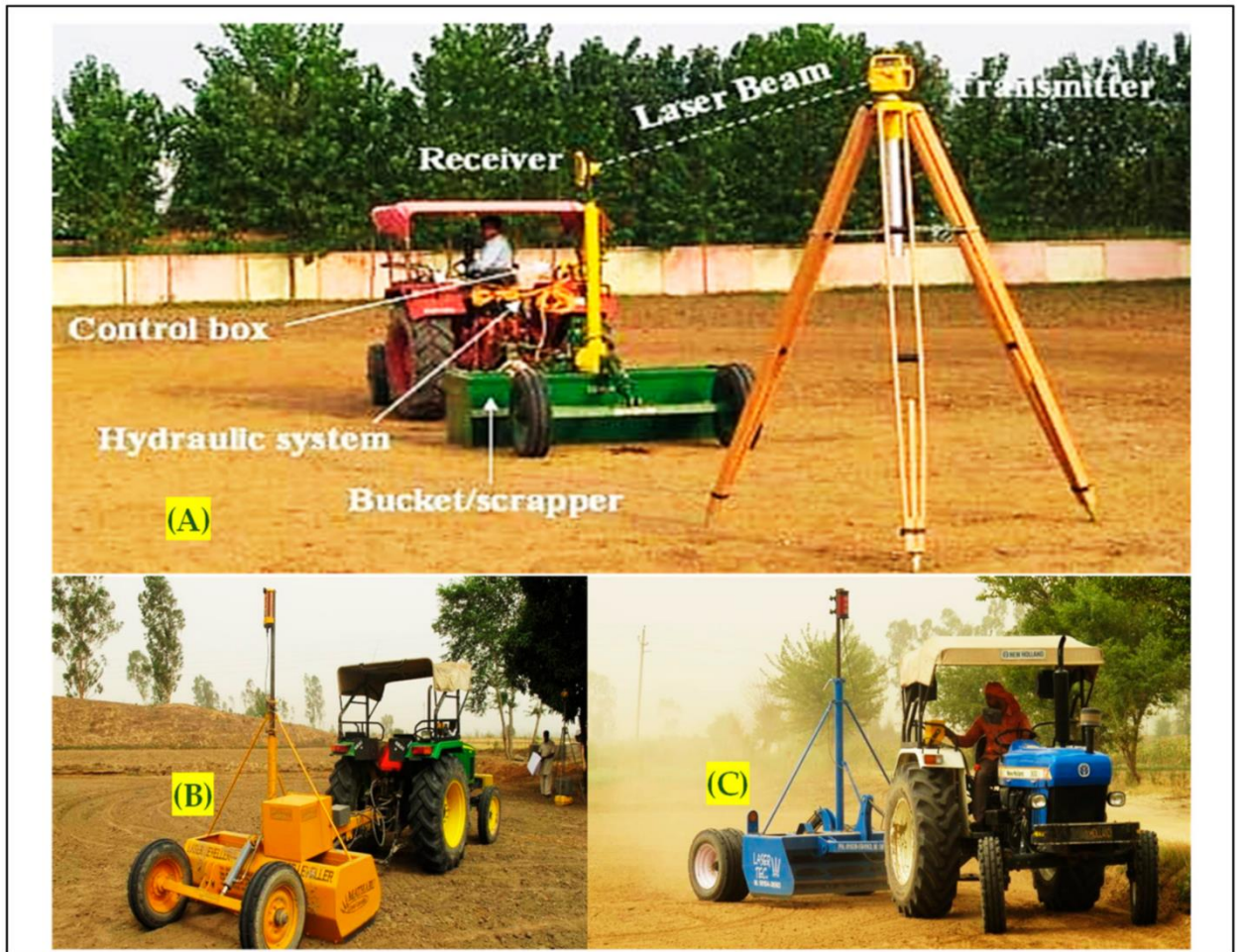
Fig. 2: Precision laser land leveling (PLL) in field conditions, (A) showing the function of different components; (B,C) PLL in operation levelling a field (Naresh et al. , 2021)
