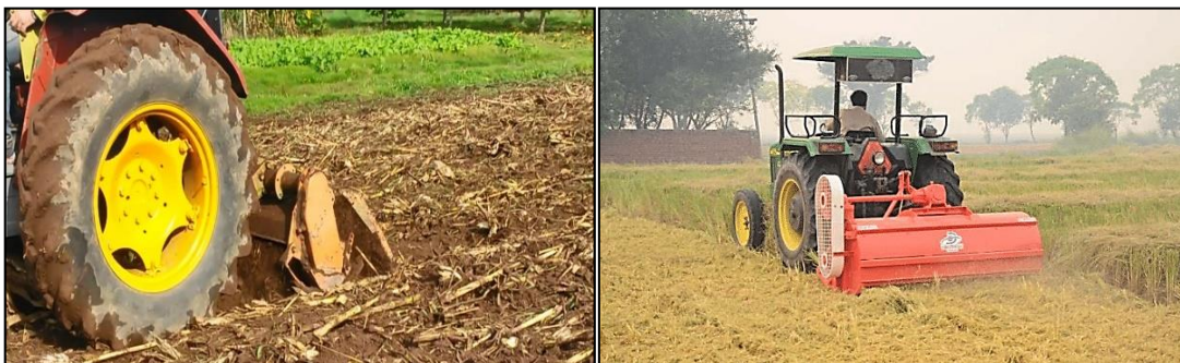
Figure 1: Residue incorporation under loose residue after harvesting of maize (left) and rice (right)
