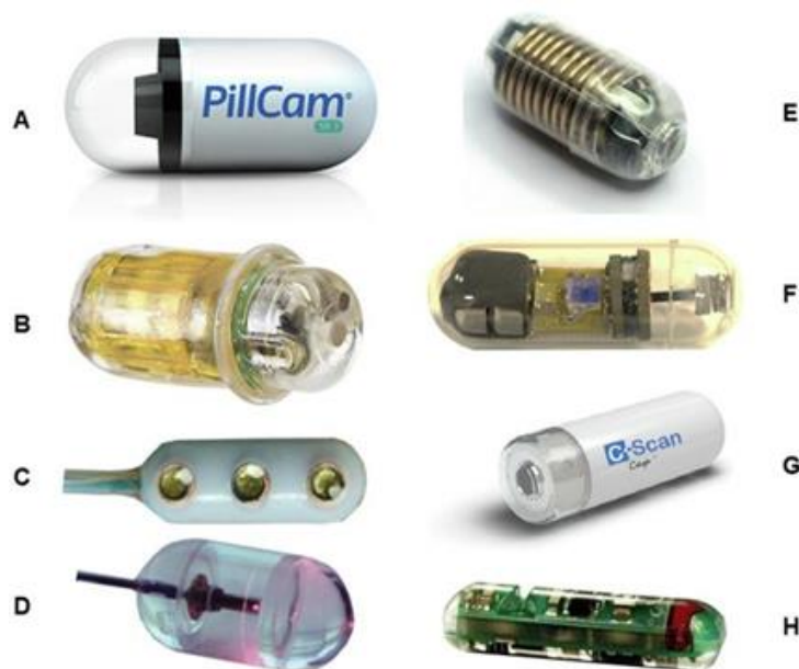
Fig. 1: Diagnostic Capsules: A) Pill Cam Capsule Endoscope (Medtronic) B) SmartPill C) Sonocap (Sonopill project, UK) D) Optical Coherence Tomography pill (OCT)(USA) E) Gas sensing Capsule F) Autofluorescence Imaging Capsule (UK) G) X-Ray Imaging Capsule H) HemoPill Optical Blood Sensing Capsule
