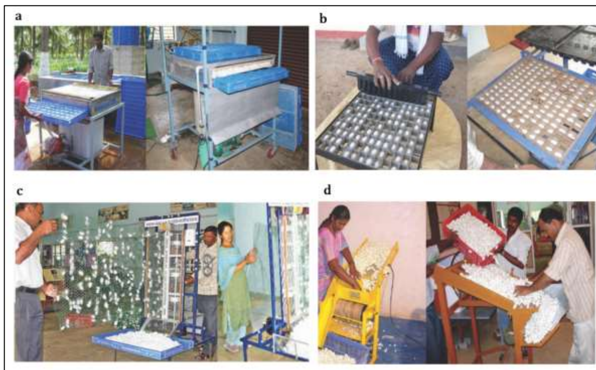
Figure 4: (a) Plastic tray washing machine; (b) Cocoon harvester for rotary mountages; (c) Cocoon harvester for plastic collapsible mountages; (d) Cocoon deflossers
