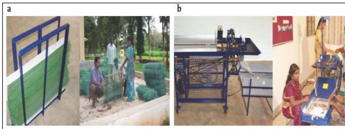
Figure 5: (a) Folding and bundling tool for plastic collapsible mountages; (b) Seed cocoon cutting machine
