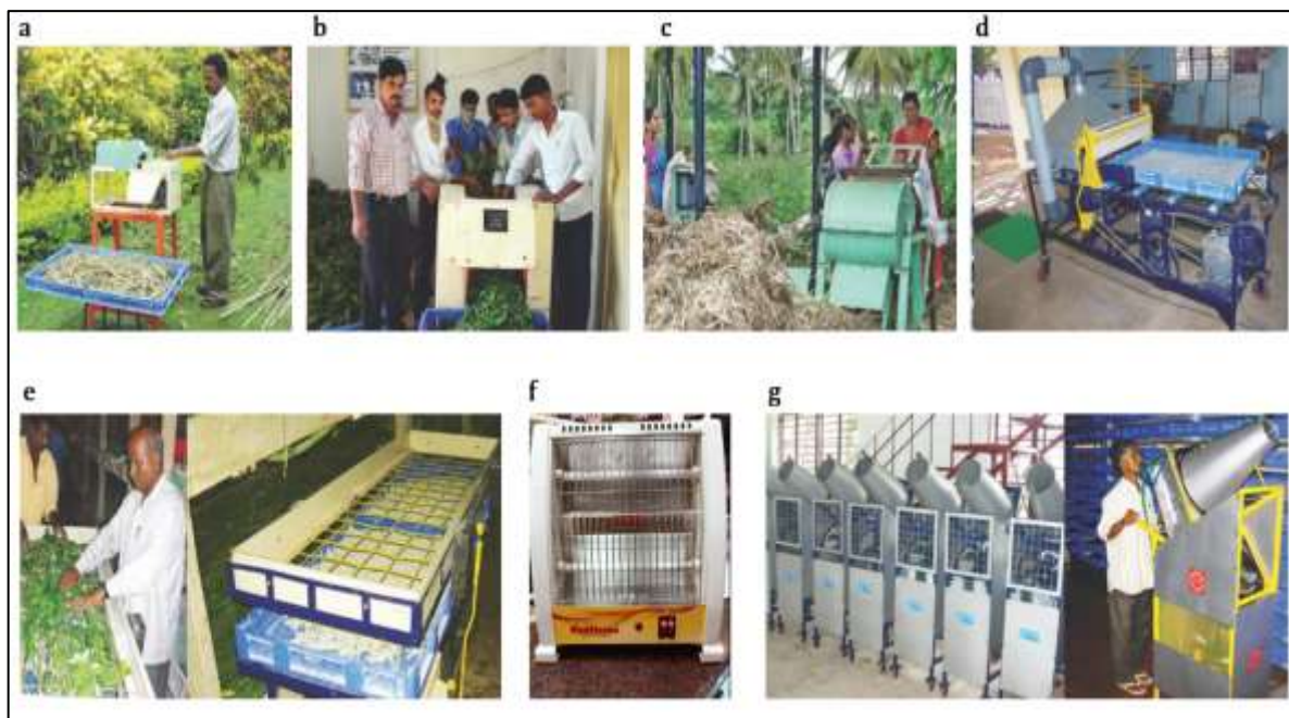
Figure 3: (a) Mulberry cutting preparation machine; (b) Mulberry leaf chopper; (c) Mulberry shoot crushing machine; (d) Disinfectant dusting machine for chawki worms; (e) Mature Silkworm separator; (f) Seri-Room Heater; (g) Seri-Humidifier cum Heater
