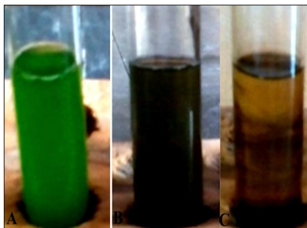
Figure 2: The colour change from green (A) to brown (B and C) during the reaction of Ag + into AgNPs due to the phytochemicals present in fruit epicarp extract of Glycosmis pentaphylla
