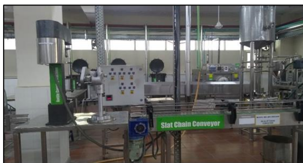
Capping & Sealing unit
