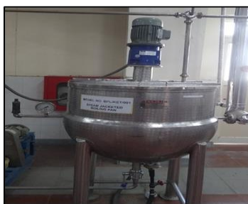
Boiling & Concentration unit
