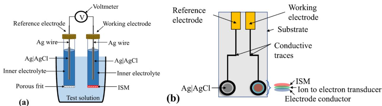
**Figure 4: (a) Schematic of a conventional ISE and (b) Schematic of a planar all solid state ISE**
