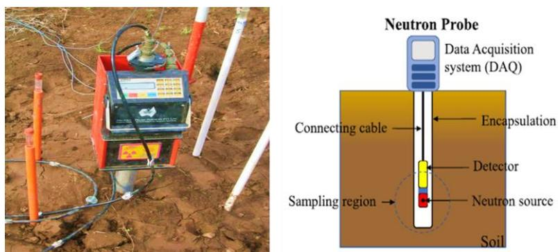
The high energy neutrons are released by the radioactive source that collide with hydrogen atom nuclei of water in soil and are captured by the detector. Neutron probes are available commercially where, with good calibration based on soil make up (metal content and density) and proper installation (sampling region completely buried in soil and minimal air gaps
