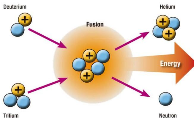
**Figure 2.15: Nuclear Fusion Reaction**
