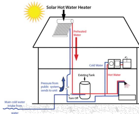
**Figure 2.8: Solar Water heater**
