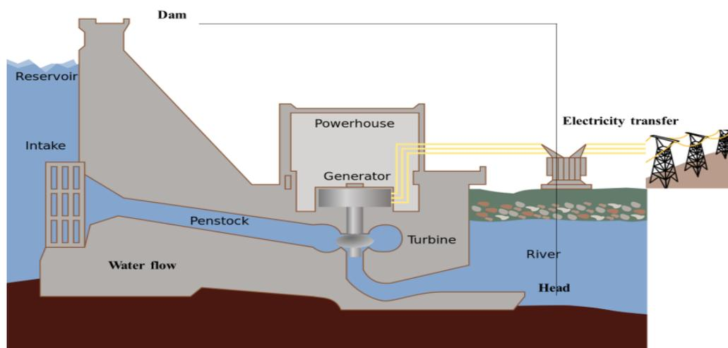
**Figure 2.9: Dam for Hydropower Generation**
