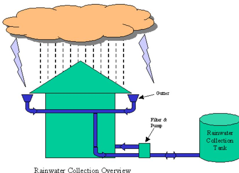
**Figure 6.2: Rainwater harvesting system**
