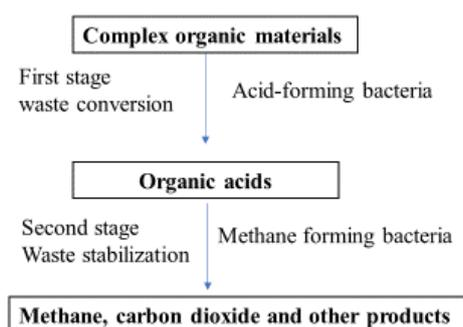
**Figure 5.2: The two phases of anaerobic digestion**
