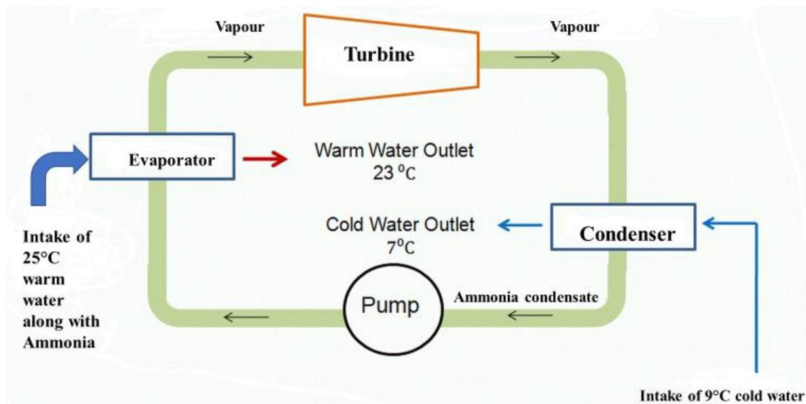
Figure 2.12: Ocean Thermal Energy Conversion (OTEC) System
