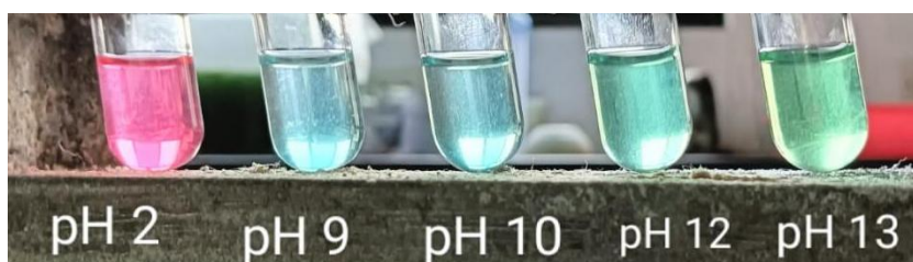
Figure 11: Ph Test result for Clitoria
