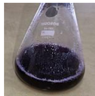
Figure 4: Pigments incorporated with binding reagent to form inks- Beetroot, Purple Cabbage and Clitoria
