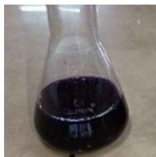
Figure 4: Pigments incorporated with binding reagent to form inks- Beetroot, Purple Cabbage and Clitoria
