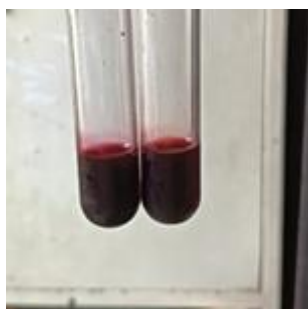
Figure 4: Pigments incorporated with binding reagent to form inks- Beetroot, Purple Cabbage and Clitoria
